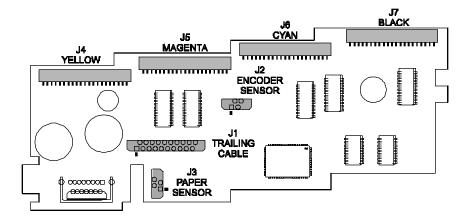
Figure 3-5. Carrier PCB Connection Locations.
